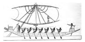
Boat of the Nile, showing how the sail was fastened to the yards, and the nature of the rigging. (Wilkinsou.)
