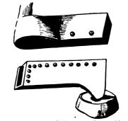
a doors. — Fig. 1. The upper pin, on which the door turned. Fig. 2. Lower pin. (Wilkinson.)
