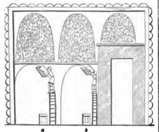
Granary, showing how the grain was put in, and that the coors a b were intended for taking it out. (Wilkinson.)
